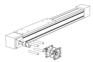
We can also put on a planetary gearbox from Wittenstein with or w/o asynchronuous motor.
